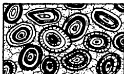
D Section of Oolitic Limestone x 20
